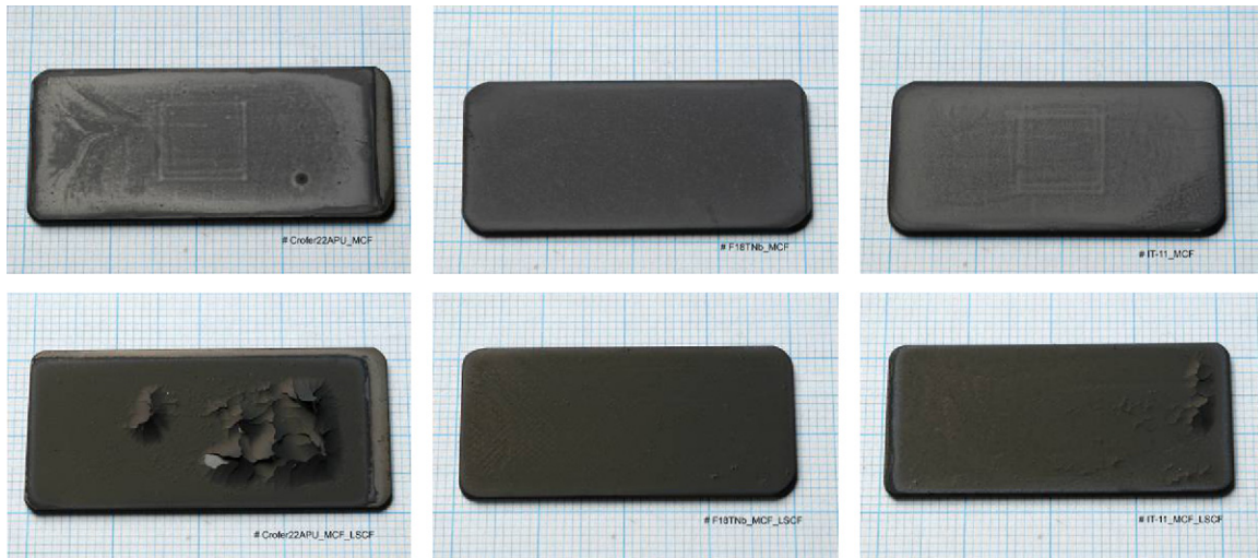
Fig. 10. Samples of Crofer22APU (left), IT-11 (right) and F18TNb (middle) coated with densified MCF (top) and coated with densified MCF and LSCF contact layer (bottom) after 1000 h of cyclic test at 800 °C in air.
